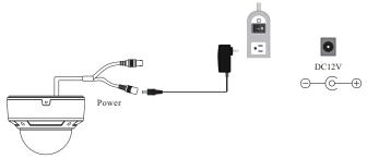
Connect the adapter to the power input connector in accordance with the camera. The recommended adapter specification for the camera is DC12V.
